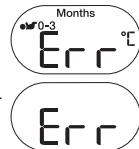
When ambient temperature is out of range (see Product Specifications below) or other system errors occur such as short or broken circuit, LCD will display "Err" to indicate system error. Red backlight on for 5 seconds.
